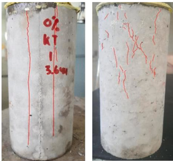
a. Normal concrete b. PET waste concrete
